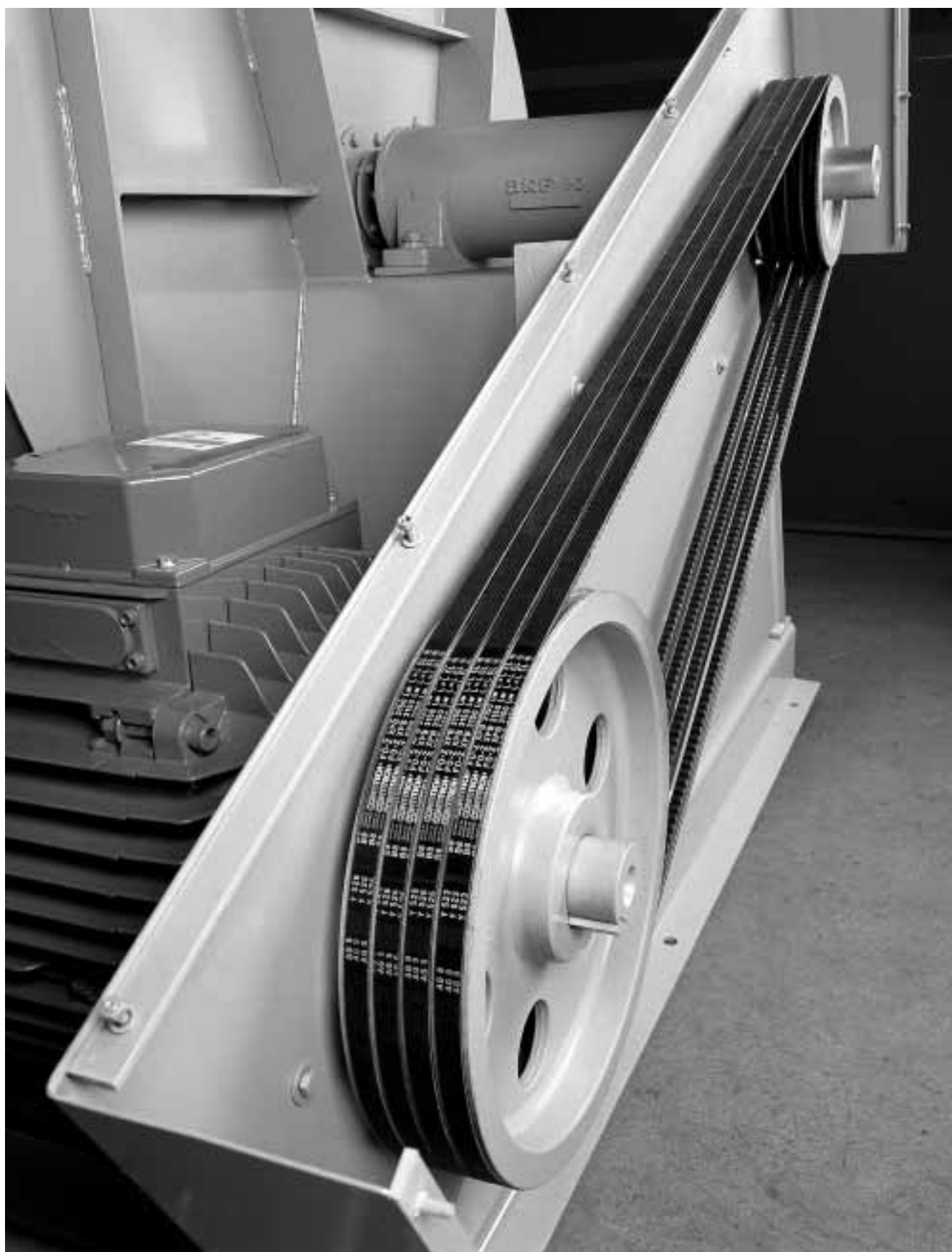
Matched-length CONTI FO® heavy-duty cogged raw edge V-belts running on a ventilator drive
